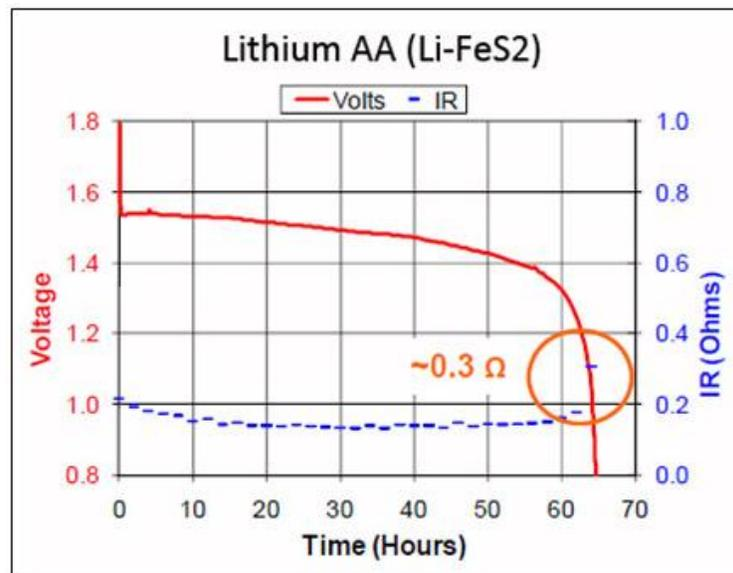
**Voltage and Internal Resistance on Discharge**
