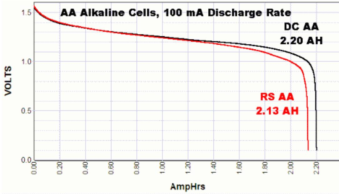
**Discharge Curves for AA Alkaline Cells**
