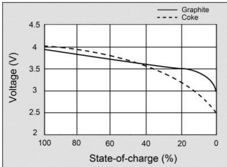
**Voltage Discharge Curve of Lithium-Ion Cell**
